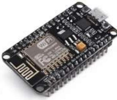
**Gambar 2. 3** NodeMCU
