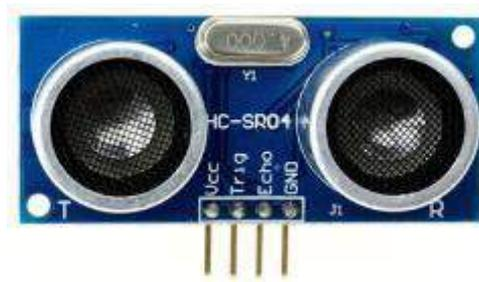
**Gambar 2. 4 Sensor Ultrasonik HC-SR04**
